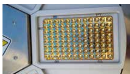
Gold-plated copper heating and cooling more quickly
