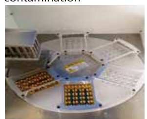
24 large capacity modules (11ml capacity perhole, suitable for large samples)
